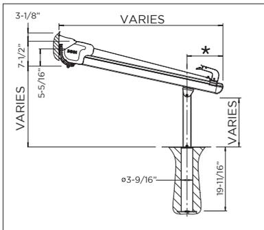
Wall mounting with ground sleeves
