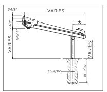
Wall mounting with ground sleeves
