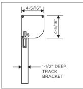
Wall Mounting w/ Direct Screw Connection
