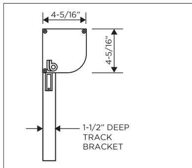
Wall Mounting w/ Direct Screw Connection
